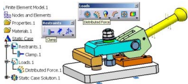
Fig. 5. Application of the fixing restraint and the loading force.
